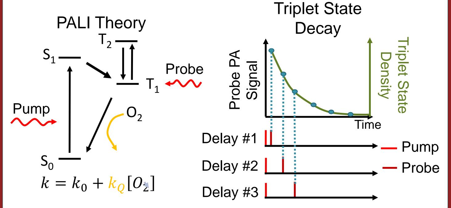
PALI "pumps" molecules to the  $T_1$  state and "probes" the number of molecules in this state by measuring the photoacoustic (PA) signal generated when T<sub>1</sub> molecules absorb the probe light. By measuring the decay over time, the decay rate of molecules from T₁ to S₀ can be calculated and used to calculate oxygen concentration once  $k_0$  and  $k_0$  are calculated using a calibration.
